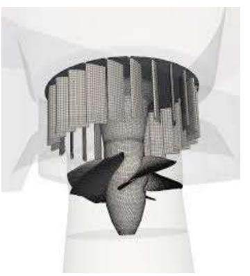
The inlet is a scroll shaped tube that wraps around the turbine's wicket gate. Water is directed tangentially, through the Wicket Gate and spirals onto a propeller runner, causing it to spin.
