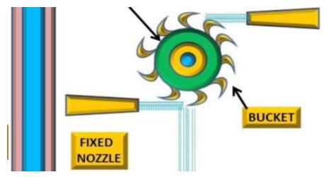
The resulting change in momentum (impulse) causes a force on the turbine blades. Impulse turbines are most often used in high head applications.
