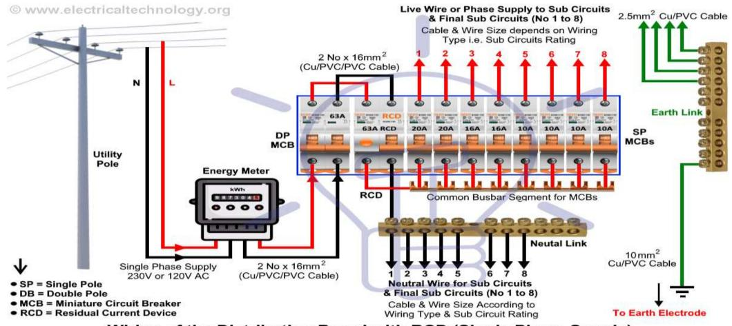
Wiring of the Distribution Board with RCD (Single Phase Supply)
